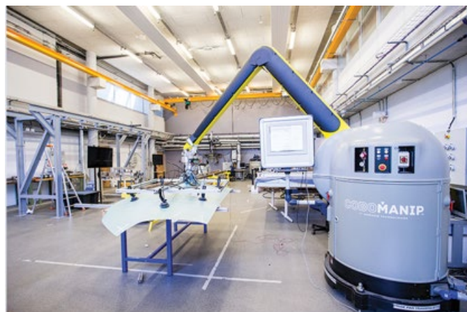
Application of Cobomanip to the handling of aeronautical structures Copyright: Cyrille Dupont
